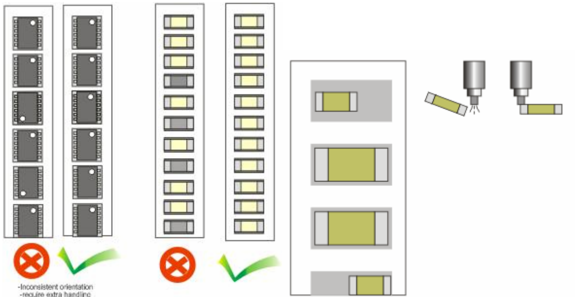
Fig 9: Repackaged parts with poor orientations and wrong tape sizes.
